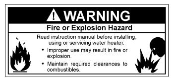
Minimum clearances between the water heater and combustible construction are 0 inch at the sides and rear, 5.5" (14.0 cm) from the front and 12" (30.5 cm) from the top. (Standard clearance.) If clearances stated on the heater differ from standard clearances, install water heater according to clearances stated on the heater.
